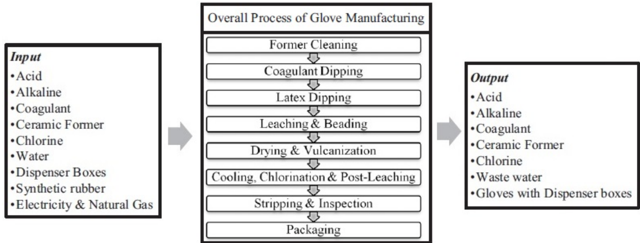
Figure 3: Simplified block diagram of rubber glove manufacturing, showing input, overall flow and output.
